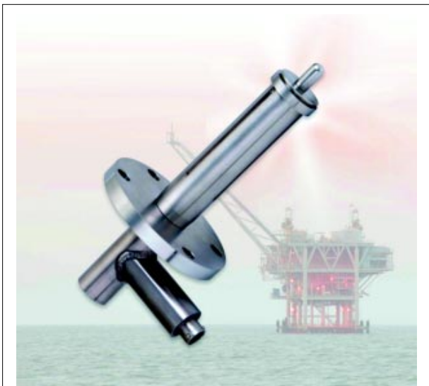
Figure B. High-pressure and seawater-resistant LVDT-based linear position sensors are incorporated into a variety of subsea measurement systems. As measurements must often be obtained in seawater to depths of 15,000 ft. and at external pressures of approximately 7500 psi, high-pressure and seawater resistant LVDT-based linear position sensors are constructed from Monel, Inconel, and Stainless Steel for pressure and corrosion resistance. These materials enhance the already high-reliability of the LVDT assembly, ensuring that it can meet service life requirements of at least 20 years, even if the device is fully exposed to seawater.
